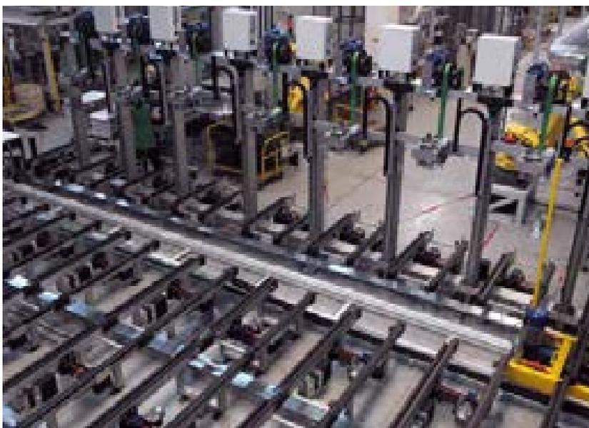
**Constant speed lines.** Traditional roller, tape, chain, belt or slat conveyor for continuous supply to workstations.
